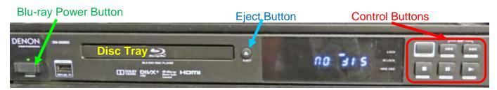
Press the **Eject** button on the Blu-ray player. When the disc tray opens, place your disc in the slot and gently push the tray back into the player. You can use either the Control Pad, control buttons on the right-hand side of the Blu-ray player, or the Denon Remote Control (aimed at the player) to control disc operations.
