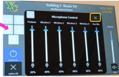
To control the microphone volume, tap the Control Panel **Audio** button to display the **Microphone** control screen. You can adjust the volume of the **Podium** microphone, **Wireless** microphones, and **Auxiliary** microphones. Tap on the **X** in the upper right hand corner of the **Microphone** control screen to delete the microphone control screen and return to the normal Control Pad functions.
