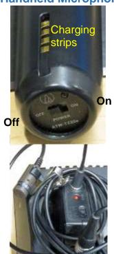
Remove the handheld microphone from the charging base and turn it on/off using the switch at the base of the microphone. A red light will indicate the microphone is turned on. To be effective, hold the microphone no more than 4 inches away from your mouth when speaking. If your head turns while
