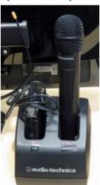
A handheld microphone and a lavalier reside in the charging base on top of the facilitator desk. Press the **Mics On** button on the control pad to project the microphones through the sound system. Note that **Power On** does not need to be on for the microphones to work! A red light underneath the label indicates that the microphones will project audio
