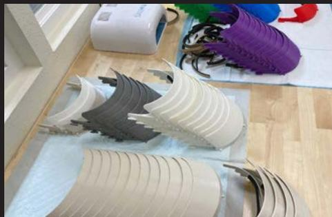
fin, CTEC’s industrial-sized 3D printer was brought online to create face shield frames in the new Fabrication Lab.
