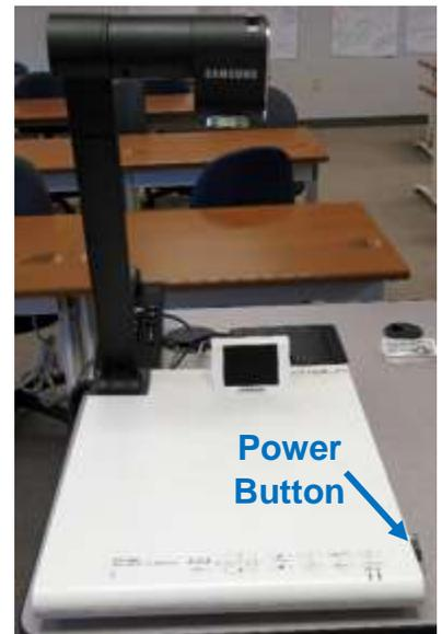
3. Rotate the document camera arm until the camera is over the object to be displayed. Then center your object/document under the camera.
