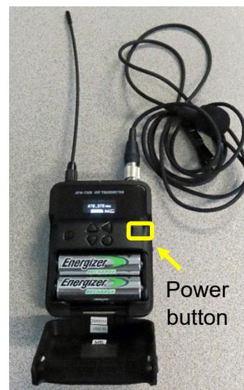
pressed, the battery charge level is displayed. One end of the lavalier cord is attached to the base and the other end has an alligator clip that holds the small microphone. Microphone placement is the key to good sound! The microphone should be attached on the sternum about 7" below the chin and slightly off-center (not directly under your mouth). Note that if mounted off-center, the speaker can't move their head back and forth while talking.
