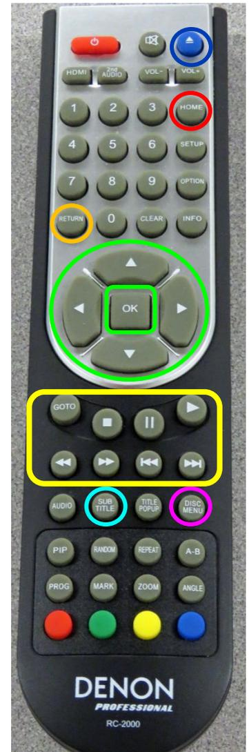
When finished playing your disc, press the **Stop** button and then the blue **Eject** button to retrieve your disc. Press the **Eject** button again to close the disc tray and change the source display back to the **Desktop PC**. Then press the Blu-ray power button to turn the player off.
