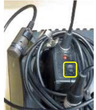
When finished with the microphone(s), be sure to turn them off and reseat them in their charging base. The 4 metal charging strips need to be aligned toward the back of the base. A red light on the charging base will blink when the microphones are charging. When fully charged, the light will remain solid red. Then tap the **Mics On** button to turn off the sound projection (the red indicator light will turn off).
